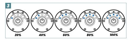
The blue battery LEDs allow you to monitor the progression of the charge.
