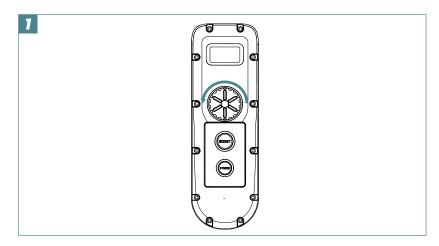
The speed adjustment dial must be at the minimum setting before you can start the Jet propulsion.
