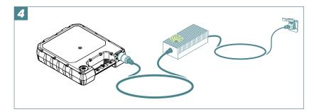
Once the battery is fully charged, all the LEDs go out and the charger indicator turns to green.
