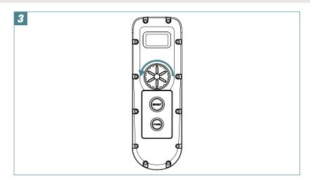
The speed adjustment dial must be put back to the minimum setting before starting the Jet propulsion again.
