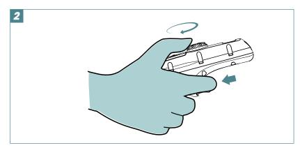
Press down on the trigger and turn speed adjustment dial to start the Jet propulsion.
