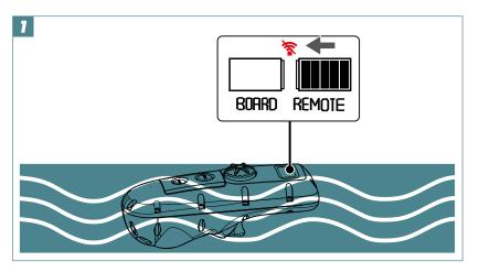
If the remote hits the water the connection and the motor will cut off.
