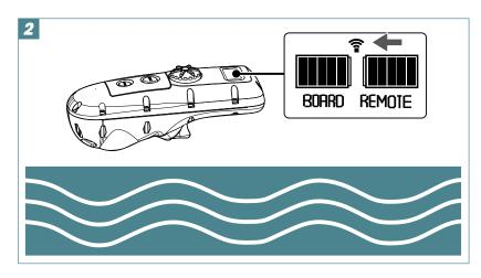
The signal automatically comes back on when the remote control is outside the water.
