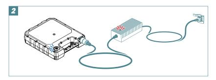
Once the battery is connected to the charger, the light on the charger should turn red.
